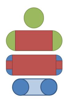
The buoyant pod geometries can be broken up into the following shapes for the purpose of volume calculation:
