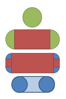
The buoyant pod geometries can be broken up into the following shapes for the purpose of surface area calculation:
