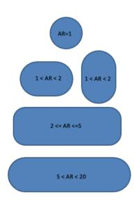
The shape of the cylindrical buoyant pods are dependant on the aspect ratio:
